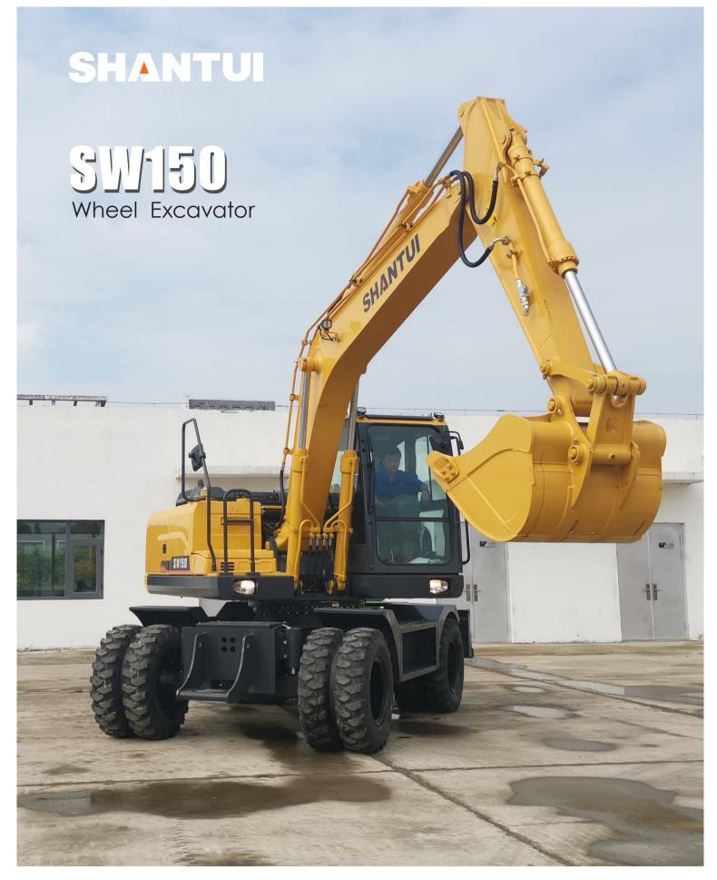
Engine Model: Gross Power: Operating Weight: WEICHAI WP4.6N 118kW/2000rpm 13500kg Flexible and Realiable
