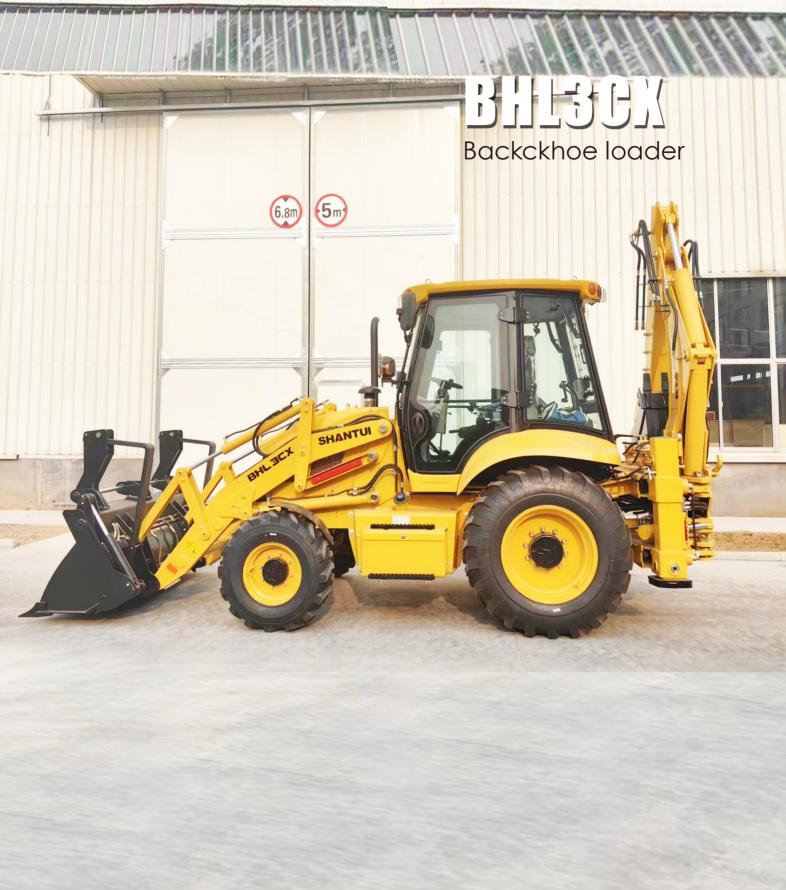
Engine Model: Gross Power: Operating Weight: Cummins 4BTA3.9-C100-II 74 kW/2200 rpm 8,200kg
